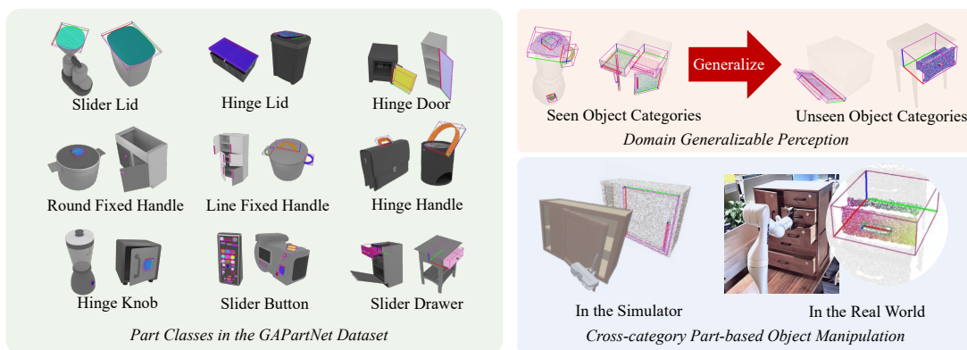
Figure 1. Overview. We propose to learn generalizable object perception and manipulation skills via Generalizable and Actionable Parts , and present GAPartNet , a large-scale interactive dataset with rich part annotations. We propose a domain generalization method for cross-category part segmentation and pose estimation. Our GAPart definition boosts cross-category object manipulation and can transfer to real.
