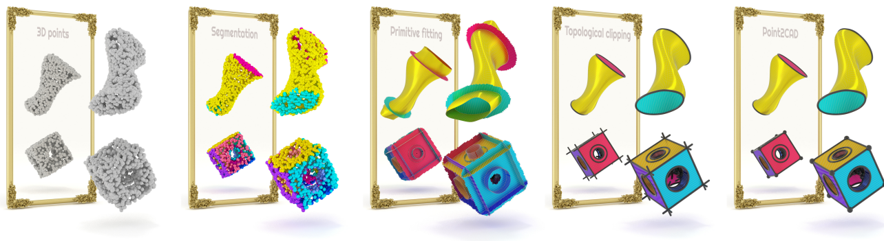
Figure 1. Point2CAD reconstructs complex CAD models from 3D point clouds. A point cloud is segmented into clusters corresponding to CAD faces. Each face is fitted with a geometric primitive or a parametric surface using a novel neural representation. Due to the analytic representation, the surfaces can be extended and intersected such that topology emerges, which is then used to clip the surface primitives.
