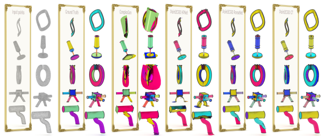
Figure 4. Results gallery. Different colors denote different surfaces. Edges and corners are depicted with black plastic. Left to right: input point cloud, ground truth mesh, and reconstruction with ComplexGen [1]. Then the proposed Point2CAD method is applied to different segmentation: with HPNet [15], ParSeNet [11], and Ground Truth. Our method reconstructs the ground truth geometry and topology from the ground truth segmentation nearly perfectly. When applied on top of pretrained segmentation modules, it outperforms the competition by a high margin.
