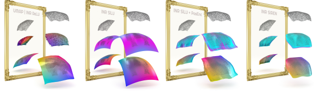
Figure 2. Inspiration items of our INR surface fitting. UMAP [7] (1 st column, middle) learns the underlying 2D manifold of 3D points along with the inverse mapping but cannot capture its smooth analytic representation. Early experiments with ReLU activations confirmed its low-frequency bias (1 st column, bottom) and piecewise linearity. SiLU [2] (2 nd column) suffers from low-frequency bias, too. We found that resolving it by adding positional encoding is challenging under our training protocol (3 rd column). SIREN [12] (4 th column) fits the data well but does not extrapolate.
